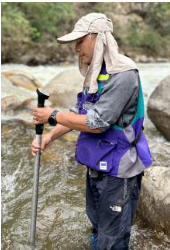
Figure 2. 3: The AVFM 6.1 Area Velocity Flow Meter used for velocity and depth. and specimens which could not be identified in the field were fixed in formalin and preserved in ethanol using specimen container. From the study sites, none of the fish samples were taken to the laboratory due to the lone fish species and the species sampled were identified on the project site. Portable water analysis testing kits was used to measure the physical parameters on site such as pH, dissolved oxygen, TDS, turbidity and temperature. For the macroinvertebrates, the materials used were A D-frame aquatic dip net with the mesh size of 600 \mu\text{m} , magnifying glass, forceps and tray. The advantages of using D-Frame dip net is because it is affordable and can be used in low gradient stream. Moreover, it is easy to handle and can be used to collect sample from more than one habitat (McIntosh et al., 2019).
