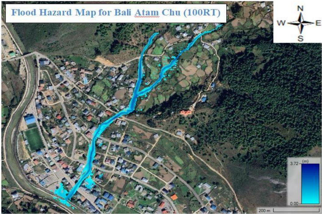
Figure 35: Flood Depth Map for Bali Atam Stream
