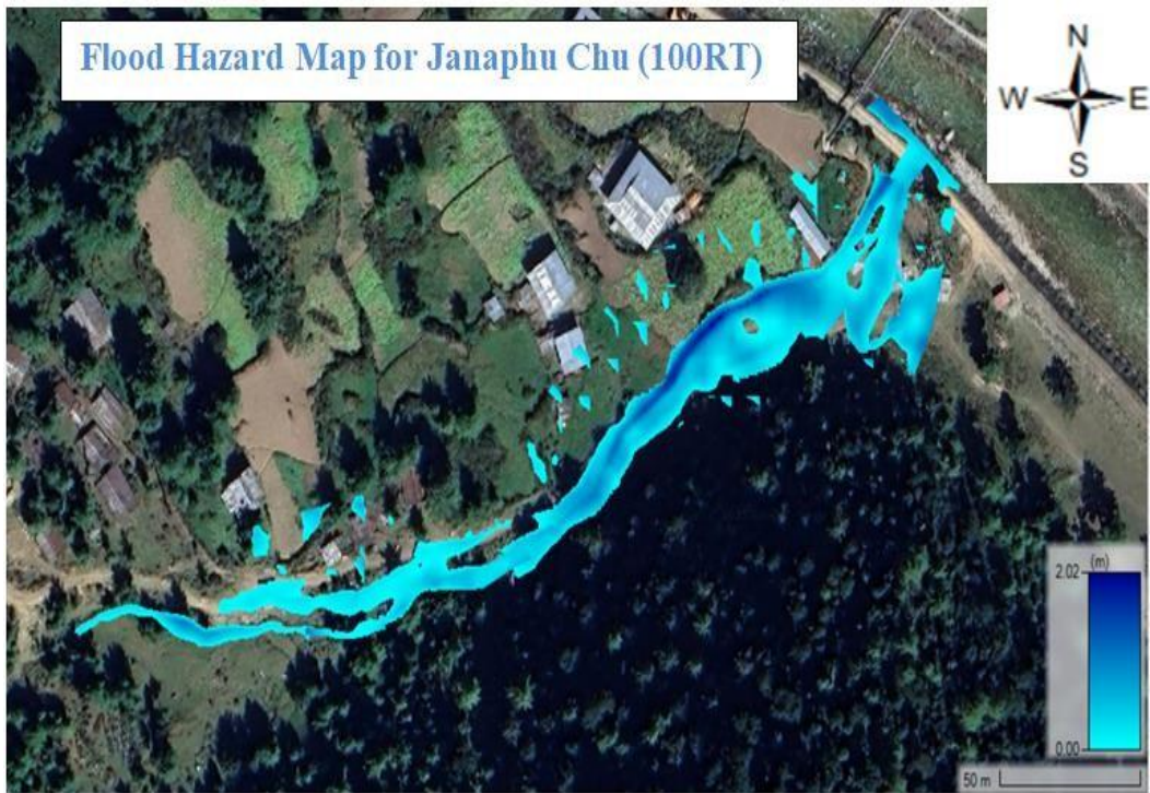
Figure 36: Flood Depth Map for Janaphuchhu Stream
