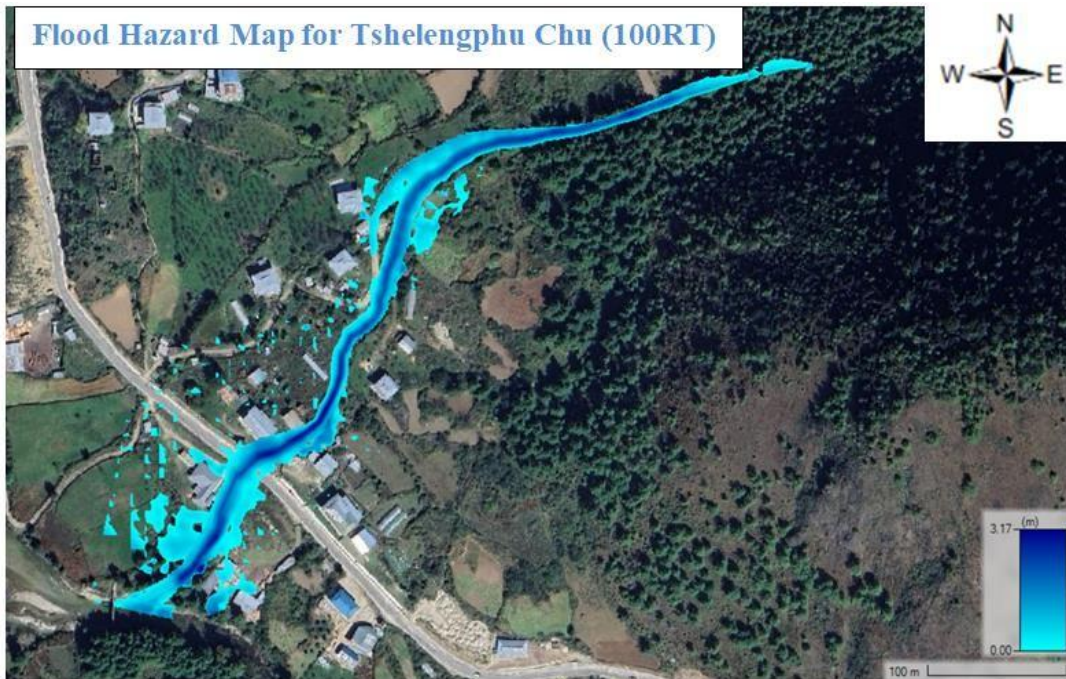
Figure 39: Flood Depth Map for Tshelengphuchhu Stream
