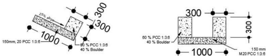
Figure 15: V-shaped and Box drain
