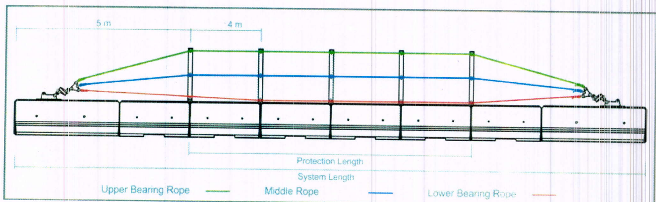
Layout of the rockfall barrier system
